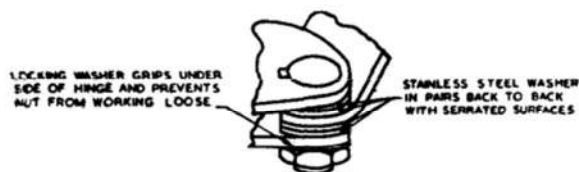
FIG. 16 ILLUSTRATION SHOWING WORKING PRINCIPLE OF FRICTION HINGES
